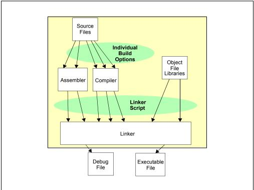
The source files are text files that are written conforming to the rules of the assembler or compiler. The assembler and compiler convert them into intermediate modules of machine code and placeholders for references to functions and data storage.
