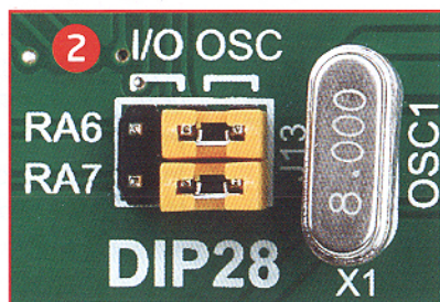
Figure 4-7: RA6 and RA7 connected to X1 quartz-crystal
